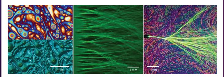
Top left: True-color interference of white light reflected from soap membrane. Bottom left: Reconstruction of membrane thickness, which maps to a refractive-index landscape. Center: Observed branched flow of light for a plane wave. Right: Observed branched flow of light when a narrow beam is launched into the membrane, forming narrow, high-intensity branches that remain focused for large distances in the disordered medium.
